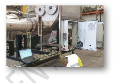
The programming of the system based upon simple control philosophy has been initiated to enable safe operation of all the relevant motors, fans, and instruments. The design of the HMI control screens has also been developed to allow ease of operator navigation, control, and operation.
