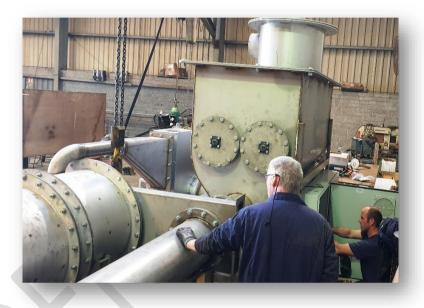
2) The Pyrotube is the location where feedstock materials are converted from their original material forms, into a biochar material. The pyrotube is a long tube, devoid of oxygen and which is heated to circa 500-600C. The pyrotube is fed with materials by
