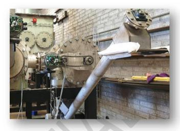
4) The combustion chamber is a high temperature furnace system that is mounted in parallel with the pyrotube. The combustion chamber has a gas burner mounted on the front end which enables the furnace to be preheated to the desired temperature. The furnace is divided into 2 chambers separated by a choke ring. The first chamber allows
